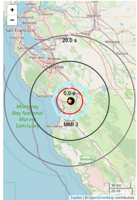
Figure 1. ShakeAlert initial earthquake location (black dot). Star is ANSS earthquake epicenter. Polygon approximates the outer range for felt ground motion. If shown, red circle is front of peak shaking when the Message was released***. Shaking takes 10 s to expand from circle to circle.
