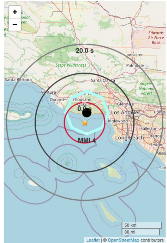
Figure 1. ShakeAlert initial earthquake location (black dot). Star is ANSS earthquake epicenter. Polygon shows estimated MMI 4 shaking intensity area. If shown, red circle is front of peak shaking when the Message was released***. Shaking takes 10 s to expand from circle to circle.
