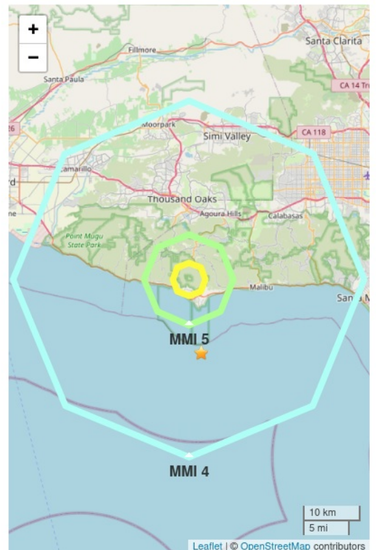
Figure 2. Polygons show shaking intensity contours for the peak magnitude estimate. Shaking of MMI 3 or less is often not felt. Star shows the ANSS earthquake epicenter.
