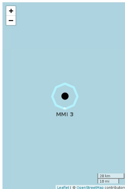
Figure 1. ShakeAlert initial earthquake location (black dot). ANSS earthquake epicenter not available. Polygon approximates outer range for felt ground motion. If shown, red circle is front of peak shaking when the message was released***. Shaking takes 10 s to expand from circle to circle.
