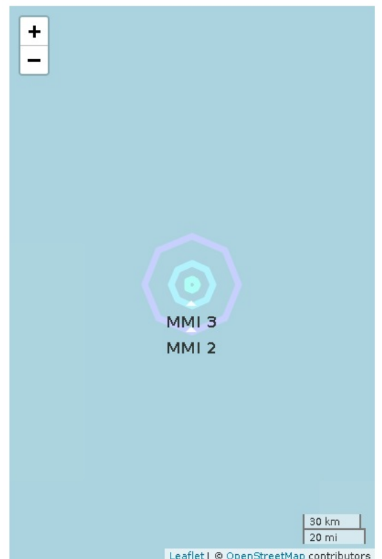
Figure 2. Polygons show shaking intensity contours for the peak magnitude ShakeAlert. Shaking of intensity 3 or less is often not felt. Regional network epicenter not available.
