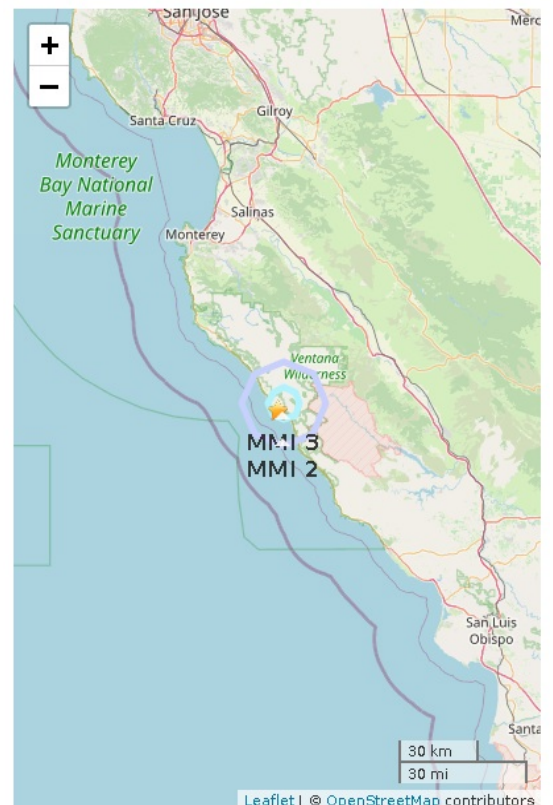
Figure 2. Polygons show shaking intensity contours for the peak magnitude ShakeAlert. Shaking of intensity 3 or less is often not felt. Star shows the regional network epicenter.
