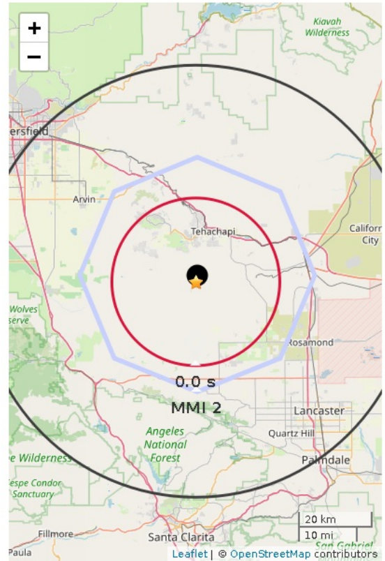
Figure 1. ShakeAlert initial earthquake location (black dot). Star is regional network epicenter. Polygon is the predicted outer range for felt ground motion (MMI 2). Red circle is front of peak shaking when the alert was released. Shaking takes 10 s to expand from circle to polygon.
