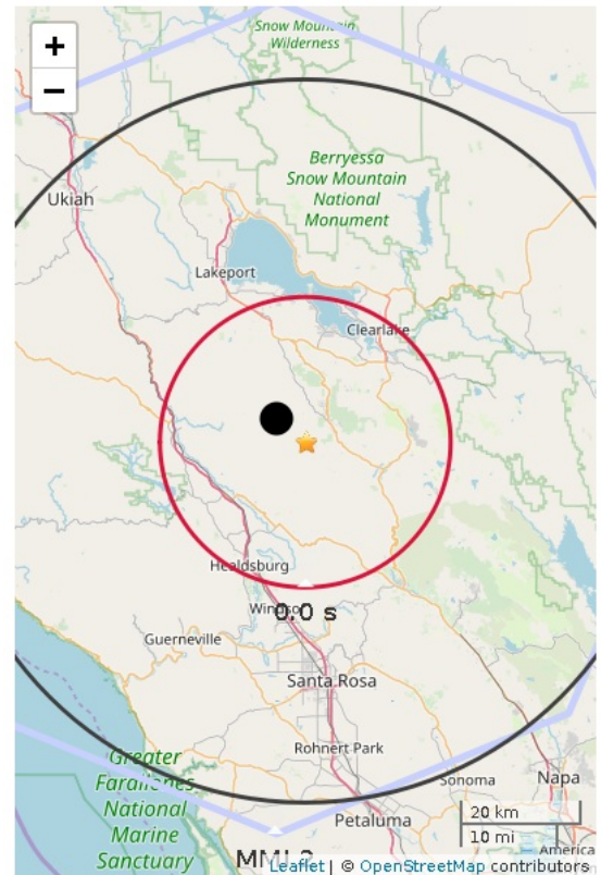
Figure 1. ShakeAlert initial earthquake location (black dot). Star is regional network epicenter. Polygon is the predicted outer range for felt ground motion (MMI 2). Red circle is front of peak shaking when the alert was released. Shaking takes 10 s to expand from circle to circle.
