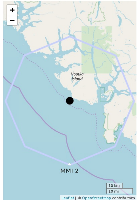
Figure 1. ShakeAlert initial earthquake location (black dot). Regional network epicenter not available. Polygon is the predicted outer range for felt ground motion (MMI 2). Red circle is front of peak shaking when the alert was released. Shaking takes 10 s to expand from circle to circle.
