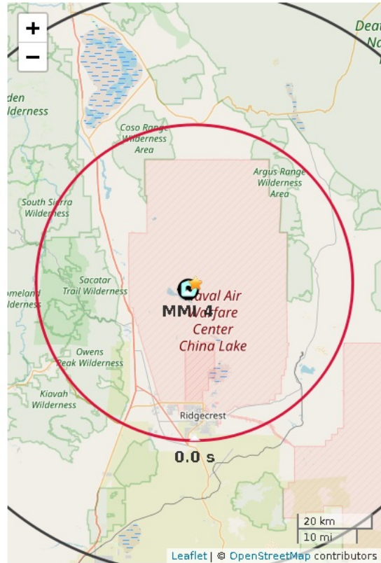
Figure 1. ShakeAlert earthquake location (black dot). Star is regional network epicenter. Polygon is the predicted outer range for felt ground motion (MMI 2). Red circle is front of peak shaking when the alert was released. Shaking takes 10 s to expand from circle to circle.
